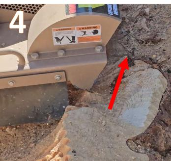
Grind side to side to remove the Bear Claw cut – Repeat steps 1-4
