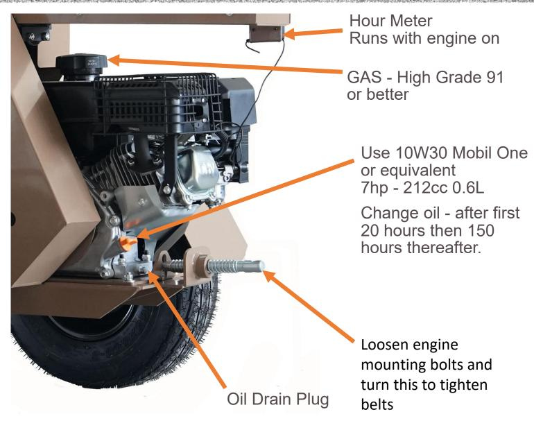
Your splitter has low oil protection. Will not start if the oil is too low, and will protect the engine
